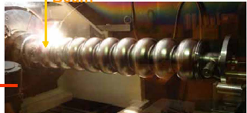
EBW of end-beam-pipes and cell-part
