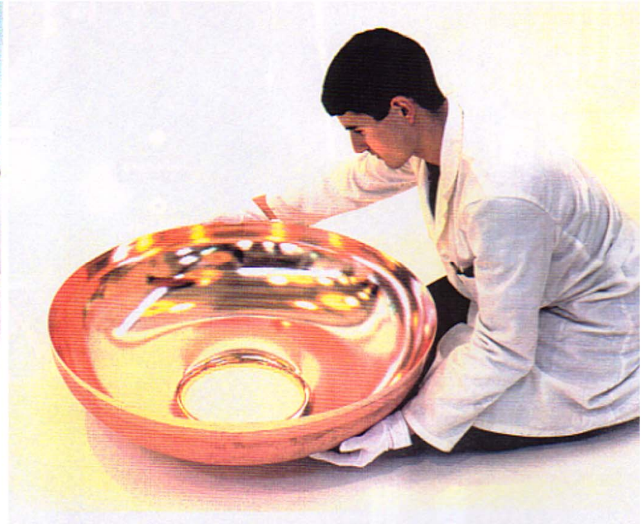
Copper half cell before Nb coating (electropolished)
