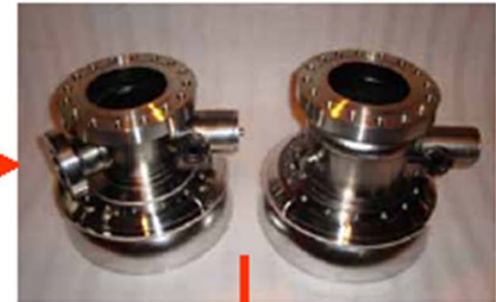
End-beam-pipes with HOM and flanges
