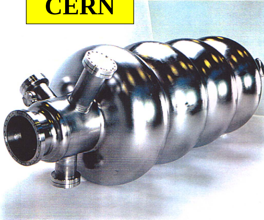
LEP-II 352MHz niobium bulk cavity
