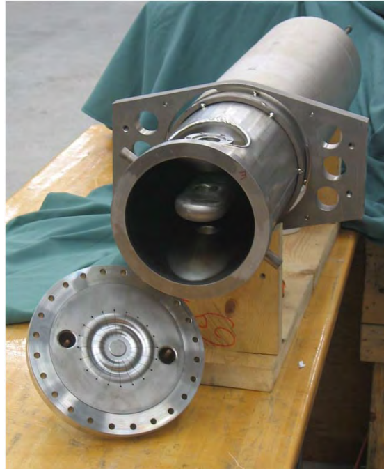
Resonator with helium vessel, tuning plate, and bottom flange
